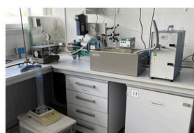
Flat-sheet membrane cells ( A = 0.01 \text{ m}^2 )
